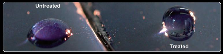
The image below shows the difference in water repellence between an untreated and treated fabric surface
